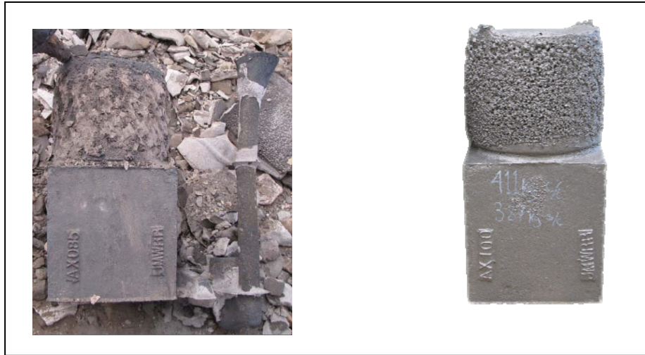
Figure 4: Before and after gouging and shot-blasting
